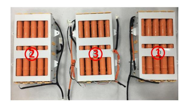
4. Install No. 3 battery box and connect the total negative power line with insulation cap. (安装 3#电池箱,并将 23 连接线一端端子固定在 3#电池箱负极处并固定拧紧,用绝缘帽防护)。
