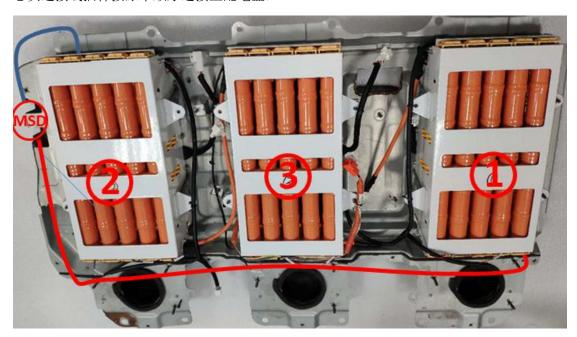
8. Connect the voltage acquisition wiring harness connector and connect the temperature acquisition wiring harness connector. (将电压采集线束、温度采集线束接插件分别进行连接)。
