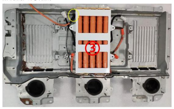
5. Install No. 1 battery case. (安装1#电池箱)。
