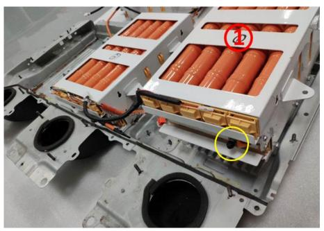
6. Install the No. 2 battery box and raise the bottom of the battery box with a wooden pad. Connect the negative terminal Harness of the original vehicle MSD and protect it with an insulating cap. (安装 2#电池箱,将电池箱底部用木头垫高,连接原车 MSD 负极端线束端子至 2#电池箱负极处,拧紧和固定,用绝缘帽进行防护)。
