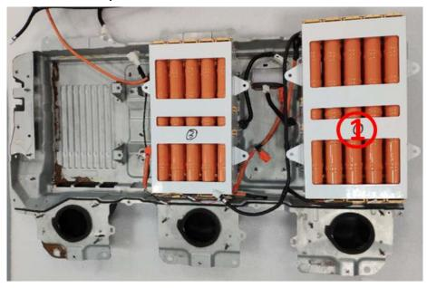
5.1 When installing No. 1 battery box, the bottom of the battery box should be padded with wood, the positive and extreme wiring harness of the original vehicle MSD should be connected, and the battery should be put into the battery box after being protected by an insulating cap. (安装 1#电池箱时: 先将电池箱底部用木头垫高,连接原车 MSD 正极端线束端子至 1#电池箱正极处,拧紧和固定,用绝缘帽防护后,安装至钣金箱体内)。
