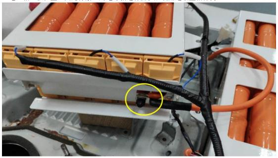
7. Fixed the box, connected the power wiring harness, installed the remaining power wiring harness into the distribution box, and connected the temperature acquisition wiring harness connector. (将1#、2#、3#箱体进行固定,将正极连接线、负极连接线分别与原车总正、总负连接线连接和固定,原车总正、总负连接线插件按原车顺序连接至配电盒)。
