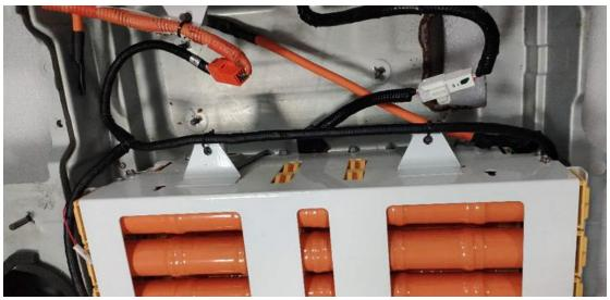
9. Put the battery pack back to the vehicle, and connect the main wire of cathode pole and anode pole in correct position. (the correct position are marked with red circle in the follow picture). (完成组装的电池组件, 放回车辆, 正确连接正负主线)。
