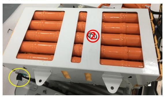
6. 1 At the other end of box No. 2, the main connecting wire of box No. 3 is tightened and fixed, and the battery is put into the battery box after being protected by an insulating cap. (连接23连接线: 将23连接线一端端子固定在2#电池箱正极位置,固定拧紧,用绝缘帽进行防护后装配进钣金箱体内)。
